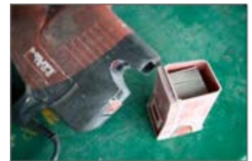
Drill with dust removal system
